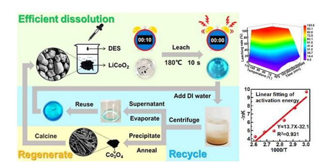
The recycling of LCO is realized in a closed-loop protocol, where the dissolution/extraction of the cobalt element involves no additional precipitates, thus enabling the reusability of the leaching solution. Credit: Journal of Energy Chemistry
