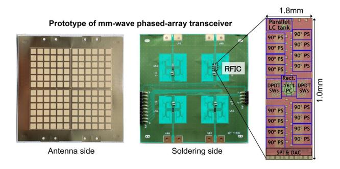
This could serve as the prototype for the transceiver. Credit: IEEE
