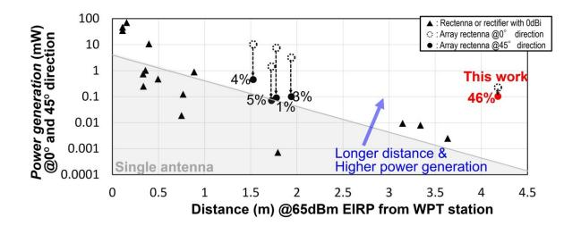
The graph demonstrates that how, as the beam steering increases from 0° to 45° during wireless power transmission, the present device can continue to generate 46% power—a much higher percentage than previous devices which would degrade to a few percent—while achieving more than twice the distance achieved by older devices. Credit: IEEE
