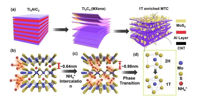
Schematic illustration of sample preparation. a Schematic illustrations of the preparation of 1 T enriched-MoS2/MXene/CNT composite through one-step solvothermal technique. The mechanism of ammonia ion intercalation induced MoS2 phase transition is shown in b–d. Credit: *npj 2D Materials and Applications* (2022). DOI: 10.1038/s41699-022-00300-0
