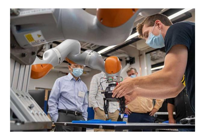
Peter Mitrano demonstrates a rope manipulation experiment. Software that he and Berenson developed can expand training data sets for challenges like rope manipulation, doubling the success rate of the robot. Credit: Dan Newman, Michigan Robotics
