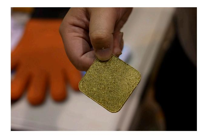
Food cement made out of dried cabbage is seen on May 26, 2022, at the laboratory of Tokyo University in Tokyo. The university's researchers Kota Machida and Yuya Sakai have developed a technology that can transform food waste into "cement" for construction use. Credit: AP Photo/Chisato Tanaka
