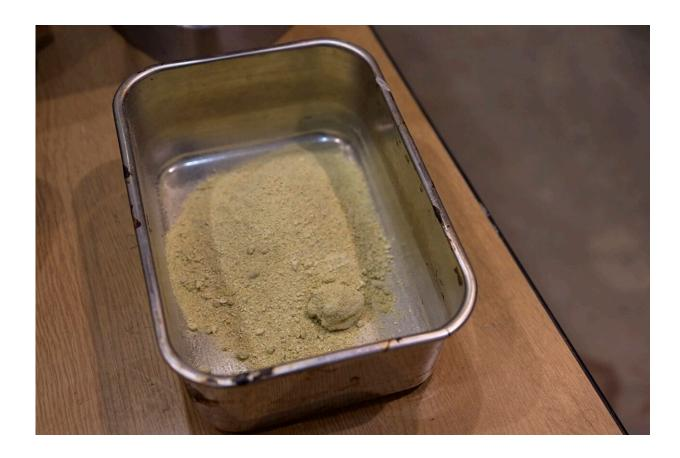
Particles of dried cabbage that were pulverized in a mixer are seen at the laboratory of Tokyo University in Tokyo, on May 26, 2022. The university's researchers Kota Machida and Yuya Sakai have developed a technology that can transform food waste into "cement" for construction use. Credit: AP Photo/Chisato Tanaka
