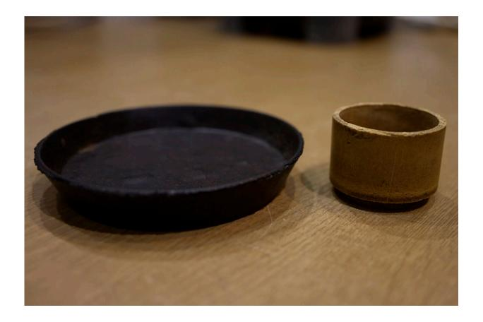
A plate and cup made from food cement are seen at the laboratory of Tokyo University in Tokyo on May 26, 2022. The university's researchers Kota Machida and Yuya Sakai have developed a technology that can transform food waste into "cement" for construction use. Credit: AP Photo/Chisato Tanaka
