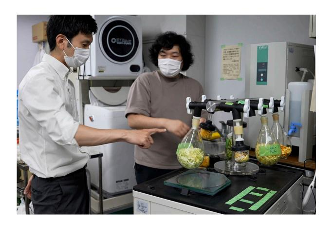
Tokyo University researchers Yuya Sakai, left, and Kota Machida, right, check on dried vegetables and fruit peels before pulverizing them to particles at their university laboratory in Tokyo, on May 26, 2022. The university's researchers have developed a technology that can transform food waste into "cement" for construction use. Credit: AP Photo/Chisato Tanaka
