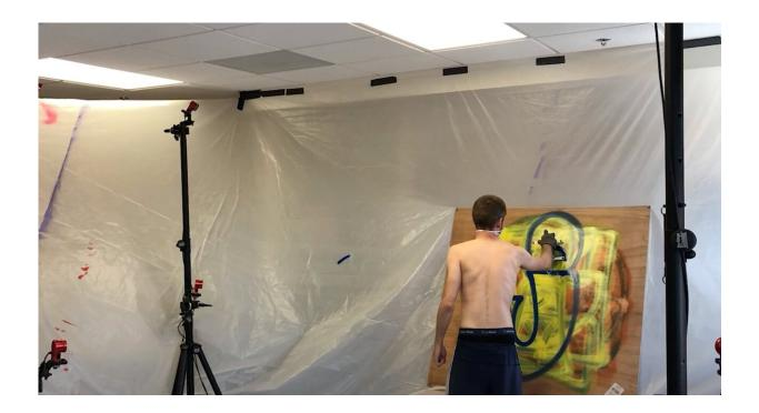
Human movement is analyzed to inform how the robot moves and paints. Credit:
