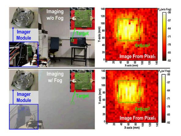
How the device can create images of a target despite heavy fog. The pixelated image on the bottom right shows the outline and shape detected through the fog. Credit: University of Texas at Dallas
