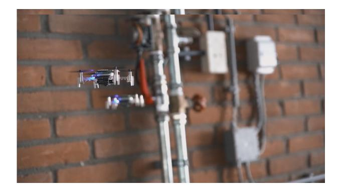
Swarm of tiny drones is able to localize gas leaks. Credit: Guido de Croon
