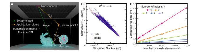
Performance of the proposed technique.(A) Schematical explanation of our twostep scattering model, adapting the BEM. (B) Correlation between trapping stiffness  $\nabla^2 U$  and the simplified form of the Gor'kov potential U', justifying the use of U' as our metric. (C) Computational performance of our acoustic holographic technique after precomputation, depending on the numbers of mesh elements (*M*) and traps (*J*). Credit: *Science Advances* (2022). DOI: 10.1126/sciadv.abn7614
