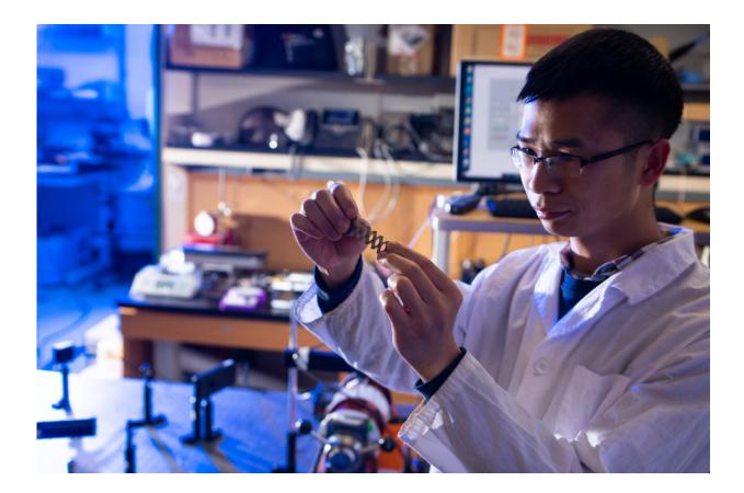
Yulong Huang, UB postdoctoral researcher in mechanical and aerospace engineering, holds a 3D-printed structure containing the magneto-ionic material used in a new study. The ability to print the material in varied shapes could facilitate different applications, scientists say. Credit: Douglas Levere / University at Buffalo
