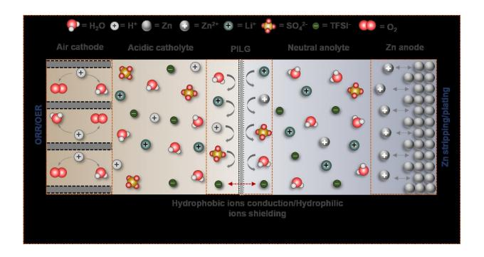
Schematic diagram of the hybrid ZAB with a proton-shuttle-shielding, hydrophobic-ion-conducting membrane, and the corresponding chemical reactions. Credit: Zhang Xinbo
