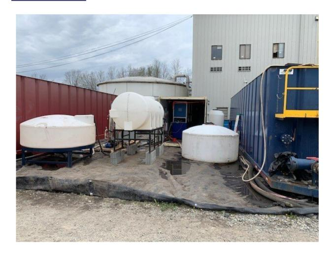
A pilot-scale membrane distillation system set up at a Marcellus Shale drilling facility in Pennsylvania. Credit: University of Pittsburgh
