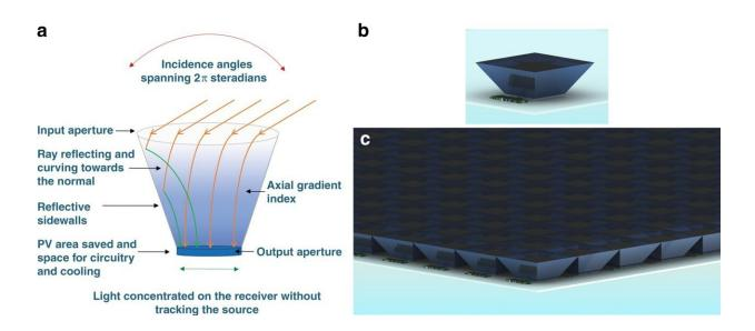
AGILE (Axially Graded Index LEns) concept and concentrator array system
