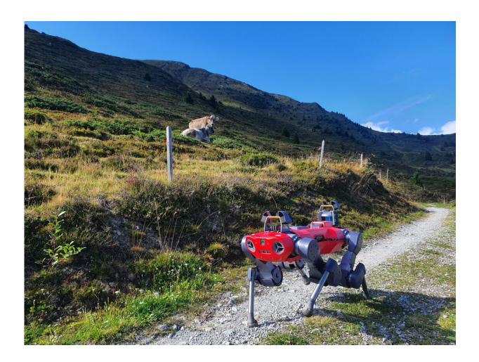
The LeMo project's dog-like robot is one of the first to have learned to walk through reinforcement learning. Credit: © ETH Zurich
