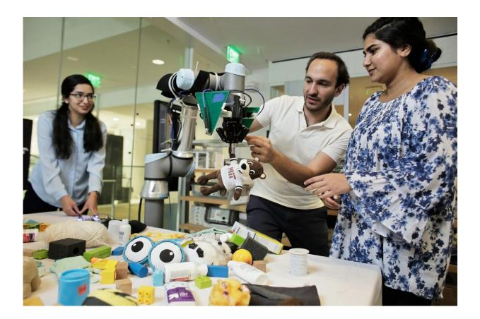
The robotic system uses radio frequency signals, computer vision, and complex reasoning to efficiently find items hidden under a pile. Credit: James Day, MIT Media Lab
