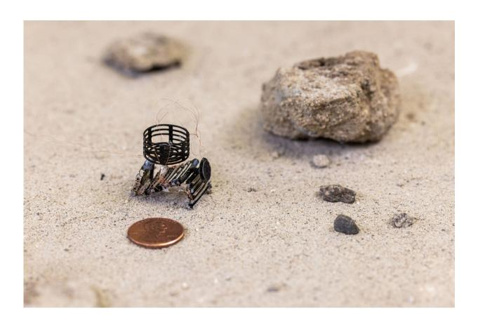
A 3D-printed "meta-bot" developed by UCLA engineers is capable of propulsion, movement, sensing and decision-making. It is manufactured all at once by a new type of 3D printing process for engineered active materials with multiple functions (also known as metamaterials). Credit: Rayne Research Group/UCLA
