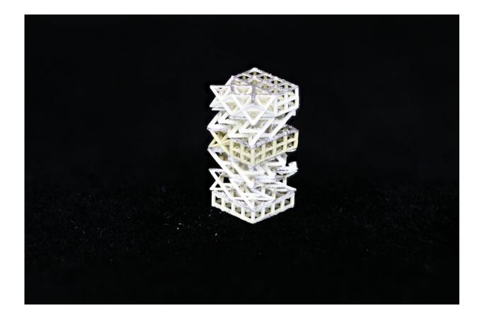
A 3D-printed lattice of piezoelectric metamaterials, which form the basis of the UCLA-developed "meta-bot." The intricate piezoelectric and structural elements
