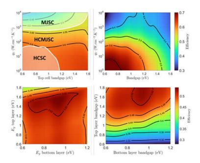
Efficiencies of the MJSC, HCMJSC and HCSC panels as a function of the bandgap and thermalization coefficient. The novel HCMJSC design, investigated by the researchers, shows higher resilience to nonoptimal bandgaps and less constrained thermalization requirements, widening the scope of candidate materials for its design. Credit: *Journal of Photonics for Energy* (2022). DOI: 10.1117/1.JPE.12.032208
