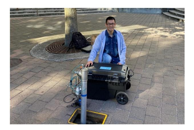
University of Canterbury Civil and Natural Resources Engineer Dr Derek Li with the sonar technology for detecting blocked and damaged underground water pipes.
