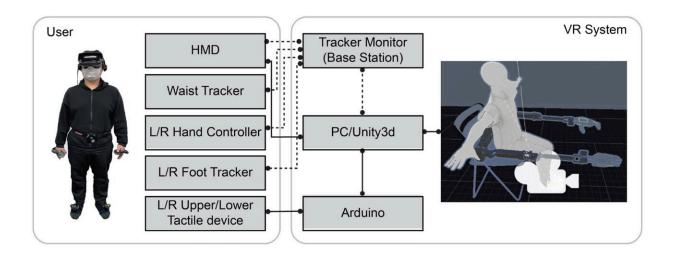
In this diagram of the system, the dotted lines represent wireless connections and solid lines represent wired connections. Credit: Ken Arai (CC BY)
