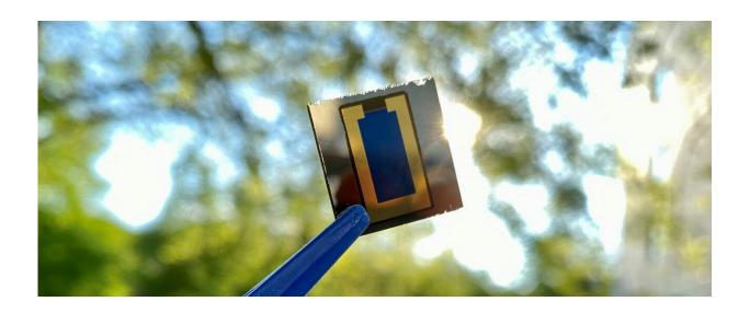
Perovskite/CIS tandem solar cells are already able to convert a relatively high fraction of incident light into electric current. Future refinements can improve efficiency further. Credit: Marco A. Ruiz-Preciado, KIT
