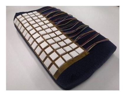
This self-powering smart pillow can track the position and motion of the head during sleep. Credit: Haiying Kou
