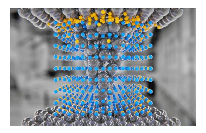
Three-dimensional schematic of a memristor made of multilayer hexagonal boron nitride. Credit: Mario Lanza / KAUST
