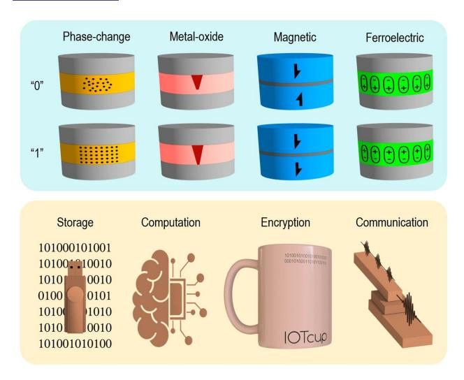
Memristive devices, in which electrical resistance can be adjusted to two or more nonvolatile levels, can be fabricated using different materials (top row). This allows adjusting their performance to fulfill the requirements of different technologies. Memristive memories are a reality, and important progress is being achieved in advanced computation, security systems, and mobile communication (bottom row). Credit: King Abdullah University of Science and Technology
