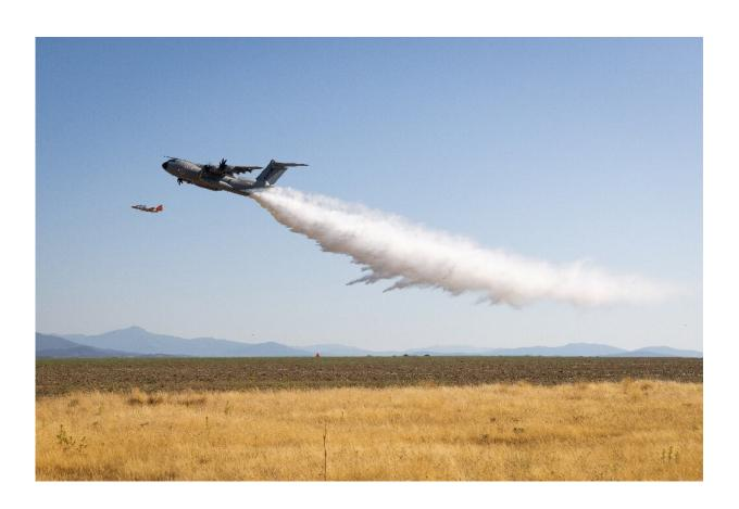
The A400M can accurately drop payloads of water at very low heights.
