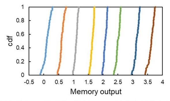
Multi-level flash memory fabricated through the technology presented in this study. As the stored electronic charge increases, the memory output between each data level can be wide enough to distinguish eight levels well.
