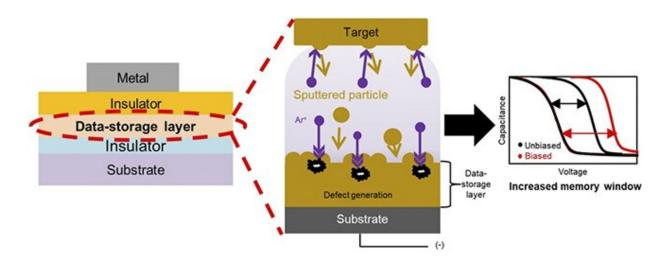
Schematic diagram of data storage increase technology of flash memory device. During the data storage layer deposition, argon plasma collides strongly to form many defects in the data storage layer. Numerous electrons can be stored in the generated defects, increasing data storage.
