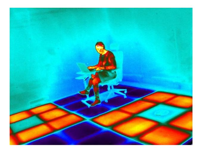
Infrared image of the modular surface heating and cooling system in the ICE climatic chamber. Credit: © D.Khovalyg, EPFL 2022
