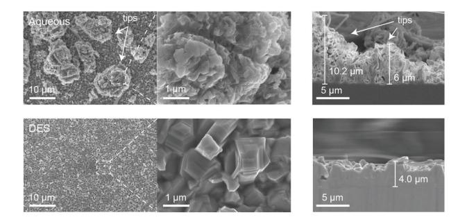
Microstructure of the surface and cross-section after electroplating of zinc. Credit: Korea Institute of Science and Technology (KIST)
