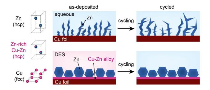
Unlike zinc particles, which are irregularly formed in a conventional aqueous electrolyte and induce corrosion, zinc grown in a DES solution is tight and uniform and maintains a stable structure even after charging and discharging in an aqueous electrolyte. Credit: Korea Institute of Science and Technology (KIST)
