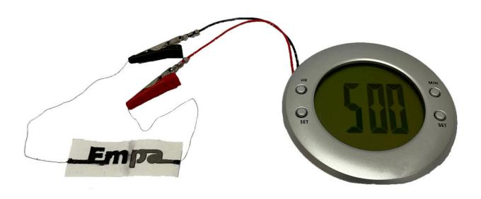
Photograph of a stencil-printed two-cell paper battery with a design that spells the name of the authors' research institution (Empa). The battery is running a liquid crystal display alarm clock. Credit: Alexandre Poulin.
