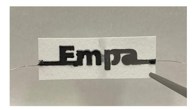
Photograph of a stencil-printed two-cell paper battery with a design that spells the name of the authors' research institution (Empa). Both of the cells are separated by a water barrier. Credit: Alexandre Poulin.
