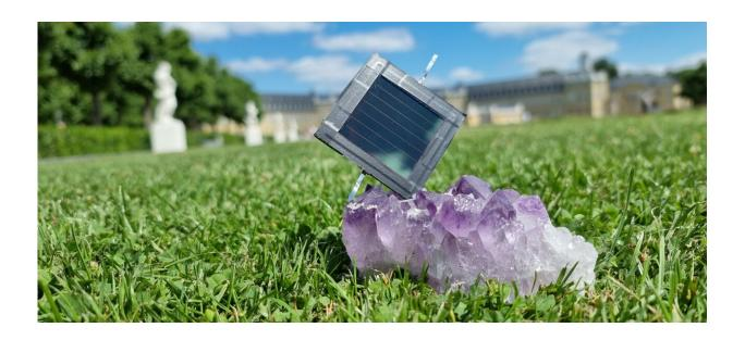
The special crystal structure of perovskites enables solar cells with high efficiency. Even more electricity can be generated in tandem configurations. Credit: Dr. Bahram Abdollahi Nejand, KIT
