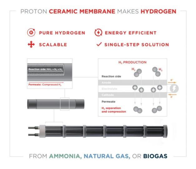
This figure shows the principles behind the new ceramic membrane used in the production of hydrogen. Credit: CoorsTek Membrane Sciences
