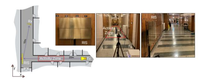
Corridor junction experiment setup. Transmitter and receiver form a virtual line of sight link via the RIS placed at the corridor junction. Dashed lines indicate the activity zone in which the experiments were perform. Credit: Muhammad Usman et al
