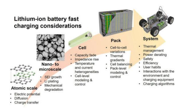
Key factors affecting Li-ion battery fast charging at different length scales. Credit: *eTransportation* (2019). DOI: 10.1016/j.etran.2019.100011
