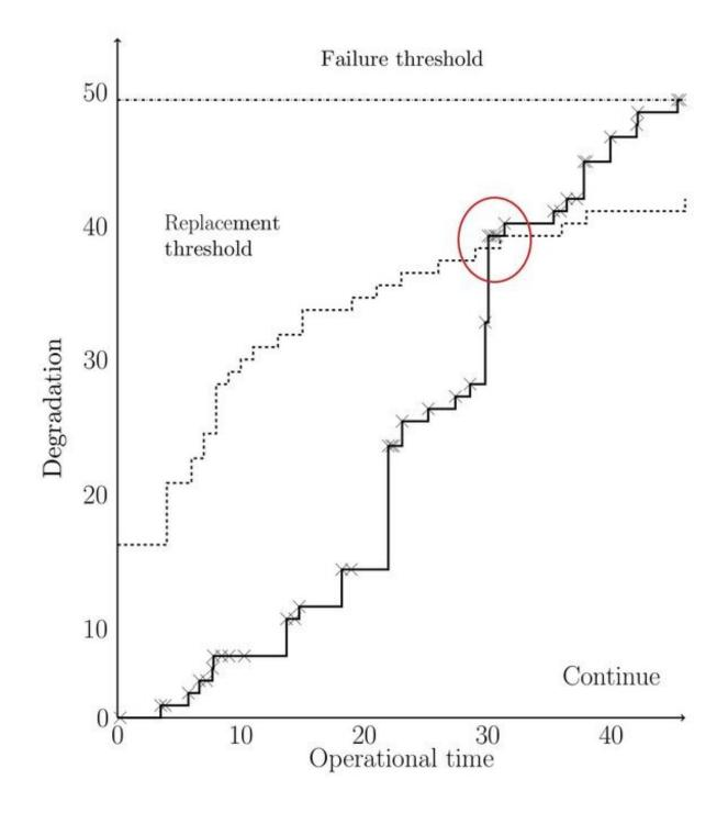
This diagram shows the aging process in time of an X-ray tube, a critical component of Philips' IXR device. Drent's combined Bayes and Markov methods predict from sensor data the optimal moment (t = 31) for replacement of the tube (the point where the dotted line of the replacement threshold crosses the degradation line). The moment is clearly below the failure threshold. Credit:
