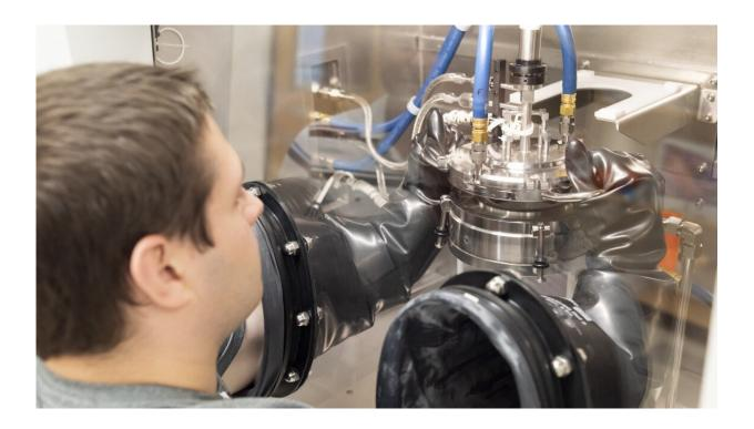
Doctoral student Cameron Gorsak opens the reactor to a metal organic chemical vapor deposition system used to create thin films of gallium oxide. Credit: Robyn Wishna
