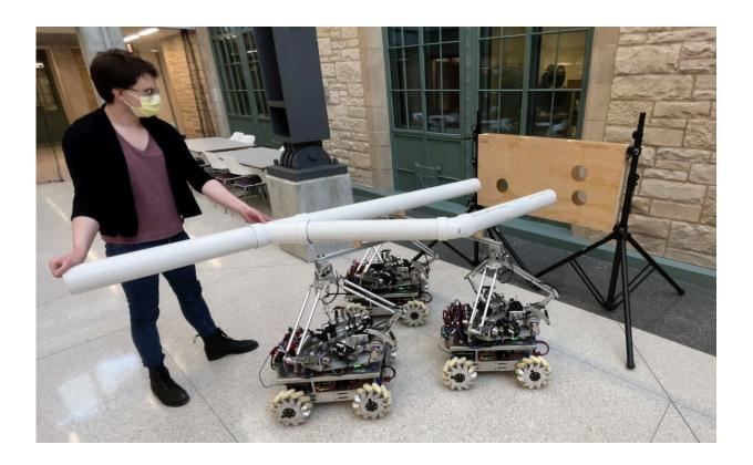
Three Omnid mocobots working collaboratively with a human on a pipe assembly task. The 16kg pipes feel weightless to the human and can be easily and intuitively manipulated due to the assistance of the Omnids. Credit: Elwin et al.
