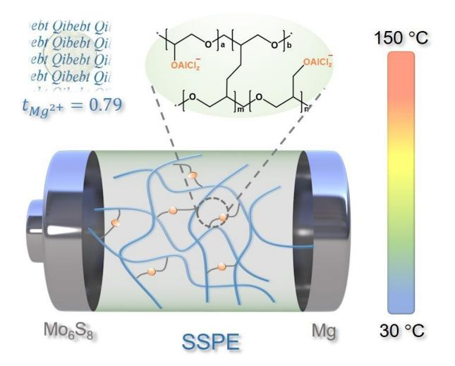
Robust self-standing single-ion polymer electrolytes enabling high-safety magnesium batteries at elevated temperature. Credit: GE Xuesong
