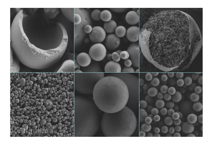
These scanning electron microscope images show silk-coated microcapsules containing vitamin C, at different scales of detail. On the left, and top center, samples made by spray drying, a method already widely used in industry. On the right and at bottom center, samples made by ultrasonic spray freeze drying, a method used by the researchers to reveal greater detail of the process involved. Credit: Muchun Liu, edited by MIT News
