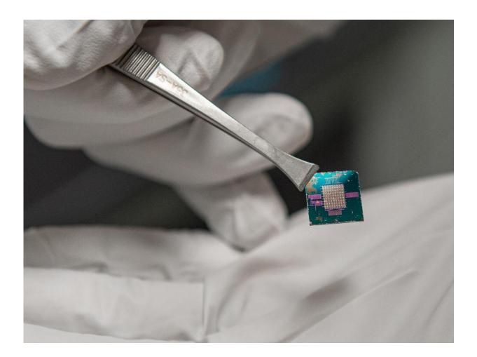
Penn State materials science and engineering researchers used molybdenum disulfide, a 2D material, to create a low-power cryptographic chip less than one nanometer thick. Credit: Kelby Hochreither/Penn State
