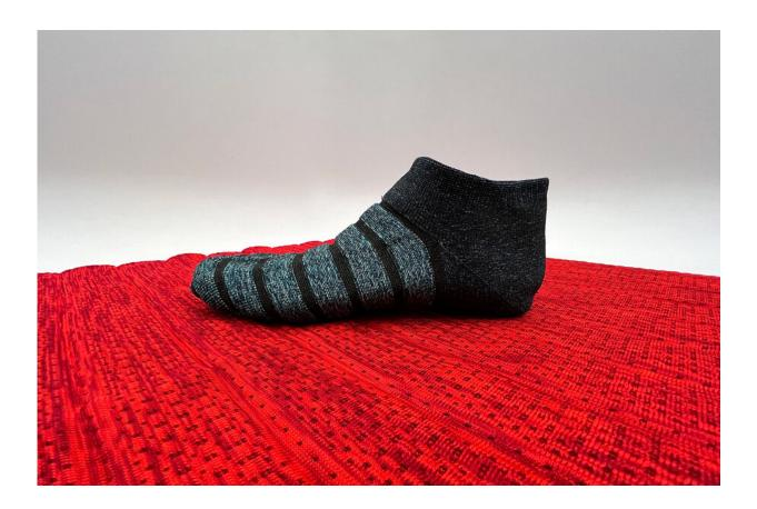
Using a novel fabrication process, MIT researchers have produced smart textiles that snugly conform to the body so they can sense the wearer's posture and motions. Credit: Irmandy Wicaksono
