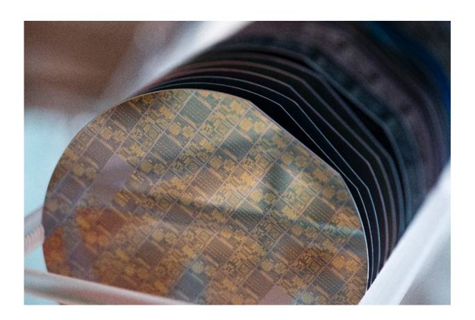
Computer chips are produced on circular 'wafers' of silicon.
