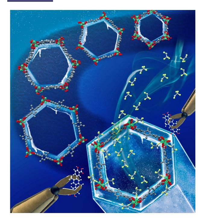
In adsorption cooling systems, molecules of vapor refrigerant (the guest) are adsorbed in the nanopores of a solid material (the host). Motkuri and his collaborators have studied how changing the geometry of the nanopores (pore engineering) and the speed of host-guest chemical interactions affect the cooling capacity and energy efficiency of adsorption cooling systems. Credit: Rose Perry / Pacific Northwest National Laboratory
