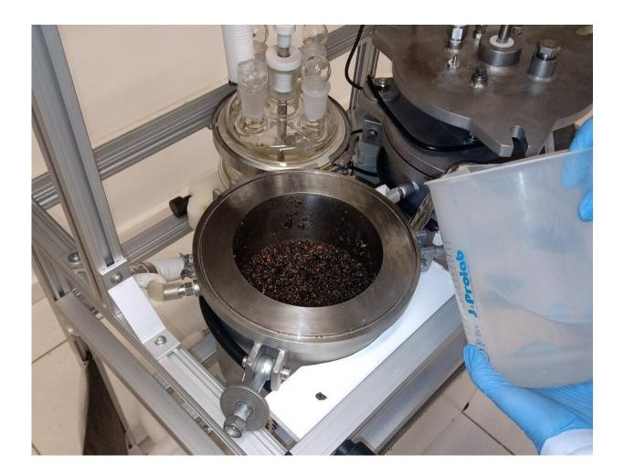
A research group at the State University of Campinas proposes treating the solid waste produced by breweries with ultrasound before submitting it to the process of digestion by microorganisms. Credit: Biotar/FEA-UNICAMP
