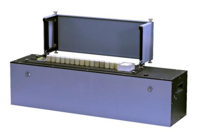
Unique experimental setup that enabled nondestructive high-precision laser measurements of thermal properties of rocks. The high-throughput apparatus works on rock samples of diverse sizes and with properties varying in a wide range of values. Credit: Evgeny Popov et al./<u>IOP Conference Series: Earth and Environmental Science</u>
