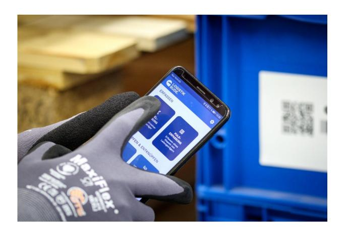
Using barcodes and the smartphone app, the current location of a load carrier is fed into Logistikbude's system. Credit: Logistikbude
