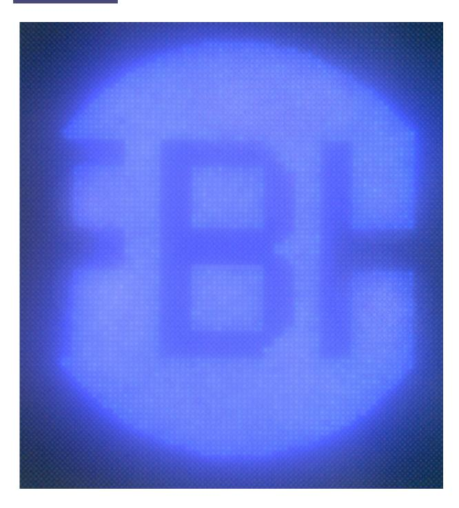
UV-luminescent pixel array of micro-LEDs with a pixel diameter of 1.5  $\mu$ m and a 2  $\mu$ m pitch shaped as FBH logo (diameter 158  $\mu$ m) under the microscope. Credit: FBH
