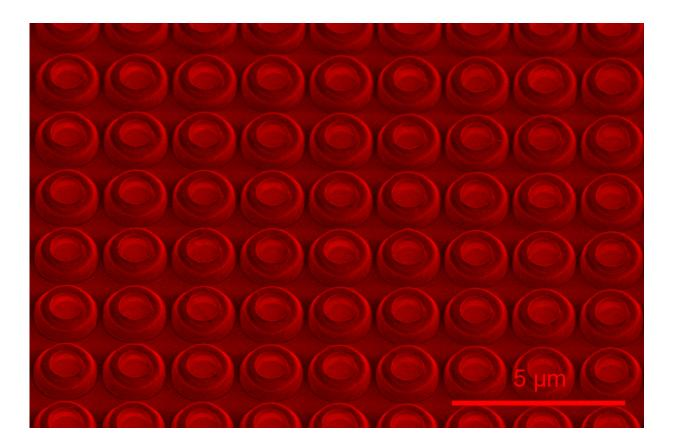
Electron micrograph of an array of UV micro-LEDs with 2 μm pitch. Credit: FBH
