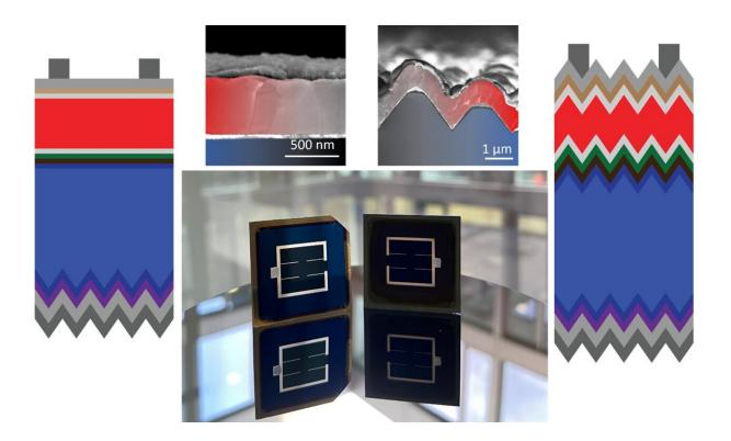
Left and right panels: Schematics of perovskite-on-silicon tandems that are either flat or textured on their front side. Upper central panels: scanning electron microscopy images of the two types of devices developed by EPFL and CSEM. Lower central panels: corresponding picture. Credit: D. Türkay, Q. Jeangros, F. Sahli, C. Wolff.
