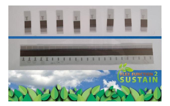
World's first organic photovoltaic cell on a film made of recycled polypropylene from drink pouch packaging material. Credit: OET Organic Electronics Technologies P.C.
