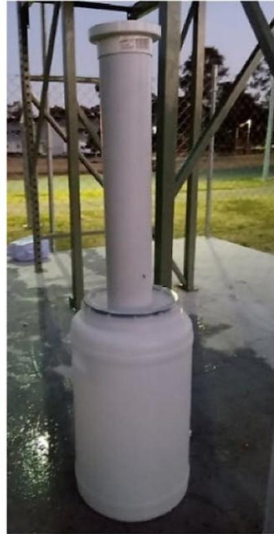
A filtration unit can be attached to an existing rainwater harvesting tank or integrated into a new system. Author provided
