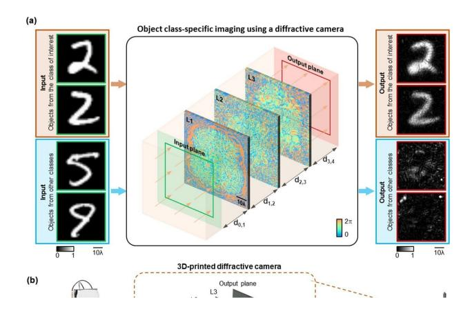
Object class-specific imaging using a diffractive camera. a Illustration of a three-layer diffractive camera trained to perform object class-specific imaging with instantaneous all-optical erasure of the other classes of objects at its output FOV. b The experimental setup for the diffractive camera testing using coherent THz illumination. Credit: *eLight* (2022). DOI: 10.1186/s43593-022-00021-3
