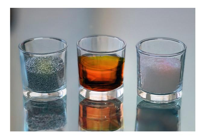
The three primary constituents of the battery are: left, aluminum; center, sulfur; and right, rock salt crystals. All are domestically available Earth-abundant materials not requiring a global supply chain. Credit: Rebecca Miller
