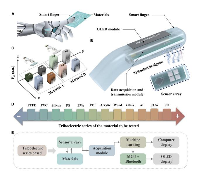
(A) Schematic diagram of the material identification process of the triboelectric tactile perception smart finger. (B) Structure of the triboelectric tactile perception smart finger, consisting of a triboelectric sensor array, data
